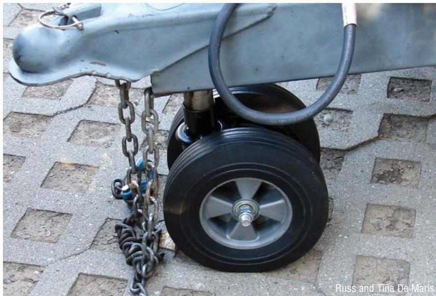
A dual-tire nose wheel can support the trailer tongue while the trailer is being moved.
