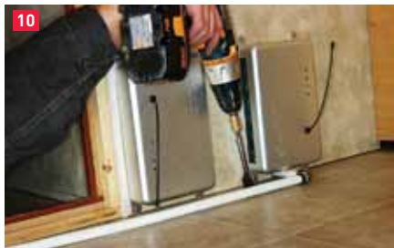
(9) After the spacing between the roller and tire has been set, the remaining bolts are tightened and torqued (40 lb-ft). (10) Two electronic control units are needed for a tandem axle installation. Here they are mounted near the batteries, and a hole is drilled in the floor to (11) route the wiring.
