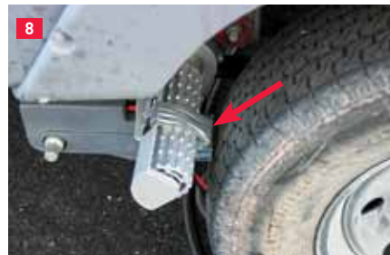
(5) With the chassis clamps in place, the crossbars can be positioned after assembling all the parts for one axle (6 and 7) and then tightened and torqued to spec. (8) Once the fit is confirmed, a 20mm spacer (not shown) is used to set the distance between the rollers and tires. Duct tape (arrow) can be used to tape the spacer to the roller during adjustment.
