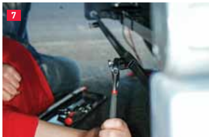
(5) With the chassis clamps in place, the crossbars can be positioned after assembling all the parts for one axle (6 and 7) and then tightened and torqued to spec. (8) Once the fit is confirmed, a 20mm spacer (not shown) is used to set the distance between the rollers and tires. Duct tape (arrow) can be used to tape the spacer to the roller during adjustment.
