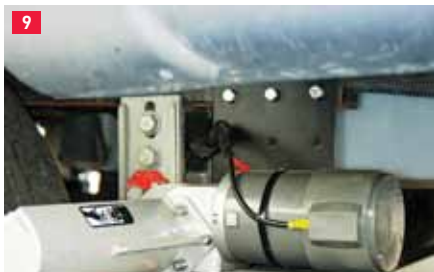
(9) After the spacing between the roller and tire has been set, the remaining bolts are tightened and torqued (40 lb-ft). (10) Two electronic control units are needed for a tandem axle installation. Here they are mounted near the batteries, and a hole is drilled in the floor to (11) route the wiring.
