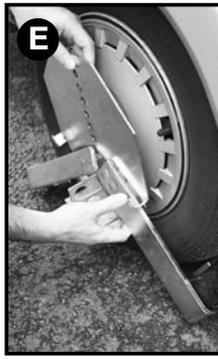
**E.** Attach the other arm into 2 of the holes in the rear plate (2). The rear plate should be positioned approximately central to the wheel face.
