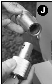
**J.** Insert the female lock portion (3b) onto the female lock portion
