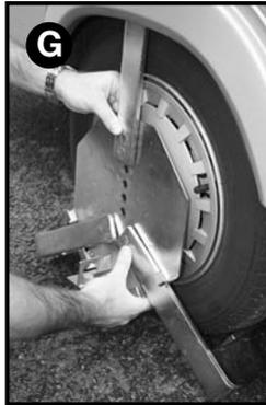
**G.** Attach the top arm (5). The arms (6 & 7) should be attached so that they rest on the ground as much as possible. To make adjustments, simply reposition by slotting the lugs into a different set of holes.
