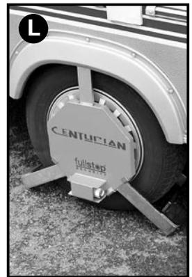
**L.** Once you are satisfied with the fit you should disassemble the wheel clamp and hammer in the security plugs (10) into the top of each hex screw. This will prevent the hex screws from being removed, using a hex key, in the event of an attack on the clamp. If the wheel clamp is to be used on a wheel with different dimensions at a later date, the security plugs can be removed by carefully drilling them out.
