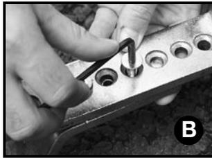
**B.** Once you have determined a suitable width insert the hex screws (8) (3 per arm) and tighten sufficiently. Repeat this procedure for the other 2 arms.
