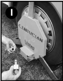
**I.** Insert the male lock portion (3a) into the apertures of the lock cradle of the face plate.
