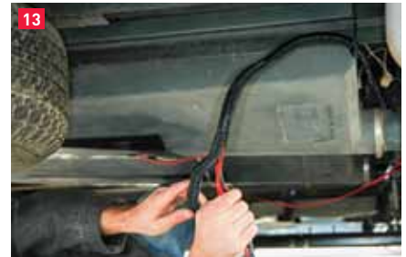
(12) With the control units securely mounted to the wall, the wires are connected to their respective terminals. (13) The kit includes split-loom conduit that is used to protect all the wiring.
